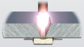
STEP 4. REMOVE BACKING TO REVEAL FINISHED BACKBEAD
